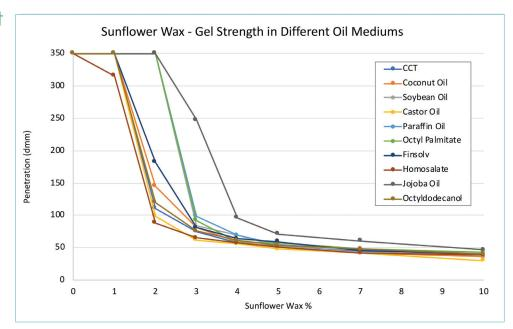
Gel strength is evaluated by measuring the distance traveled by a cone once its vertex pierces the surface of that gel; this is measured in increments of 1/10mm. When reading a gel strength graph, remember the results are inverse. The lower the value the harder the gel, and the higher the value the softer the gel.
